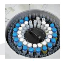
Locker design for reagent/sample disk rotation 40 positions for reagent, compatible with Olympus and Hitachi bottles
